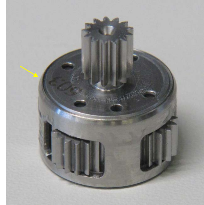
Radial swaging between planetary-carrier-sun-gear and cage to eliminate welds & adhesives
