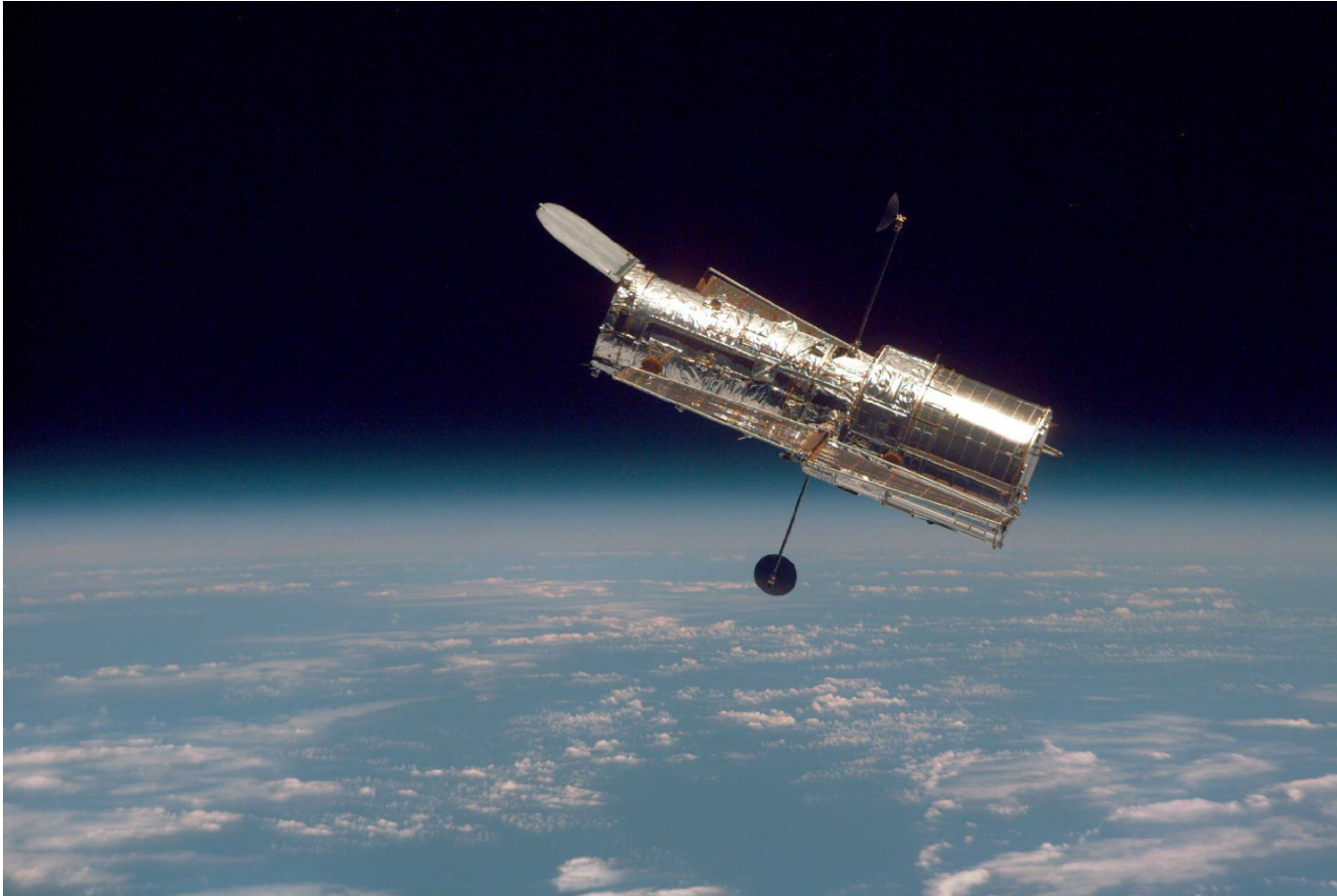
Hubble Space Telescope (HST) – 2.4 meter mirror
